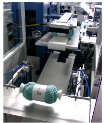
Automatic hand-over to packaging machine
